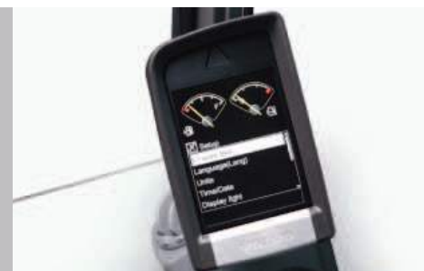
Hammer & shear: variable flow and pressure pre-setting
